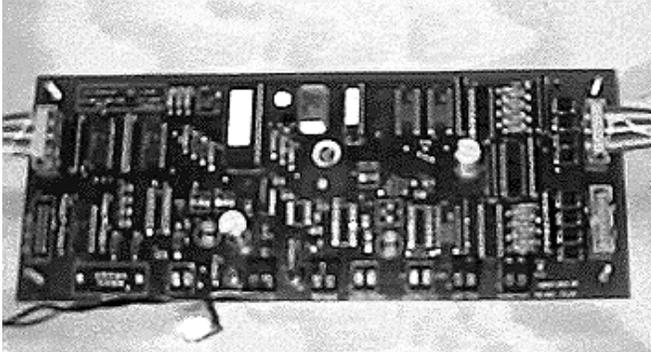
Connecting your Graphic Display Annunciator to other systems usually requires an interface between the output signals of the driving system and the graphic display lamps. Many times the interface is unique to the driving system, so a unique interface has to be designed. In some cases, additional features such as lamp tests, audible alarms, etc., must also be added, which complicates the interface.
